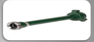
The lightweight pup joints with integral wing union end connections enable faster, easier makeup and break-out of temporary flow lines than ever before. Available in lengths up to 12 feet, these alloy-steel pup joints efficiently handle a complete range of well servicing <u>fluids at cold</u> working pressures up to 15,000 psi. pup joints are also available for sour gas services at working pressures up to 10,000 psi
